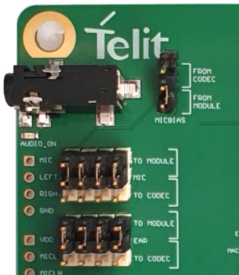
Figure 39: Jumpers Configuration for Audio in Analog Mode
