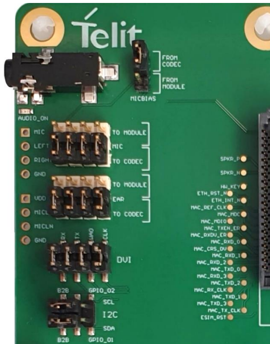
Figure 38: Digital Audio Jumpers Configuration
